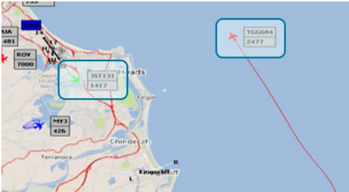
Figure 13: Conflict between Jetstar (JST) Flight 131 departing for Auckland and Tiger (TGG) Flight 604 arriving from Sydney, requiring JST131 to depart Gold Coast on runway heading (4 December 2019). Source: Airservices WebTrak
