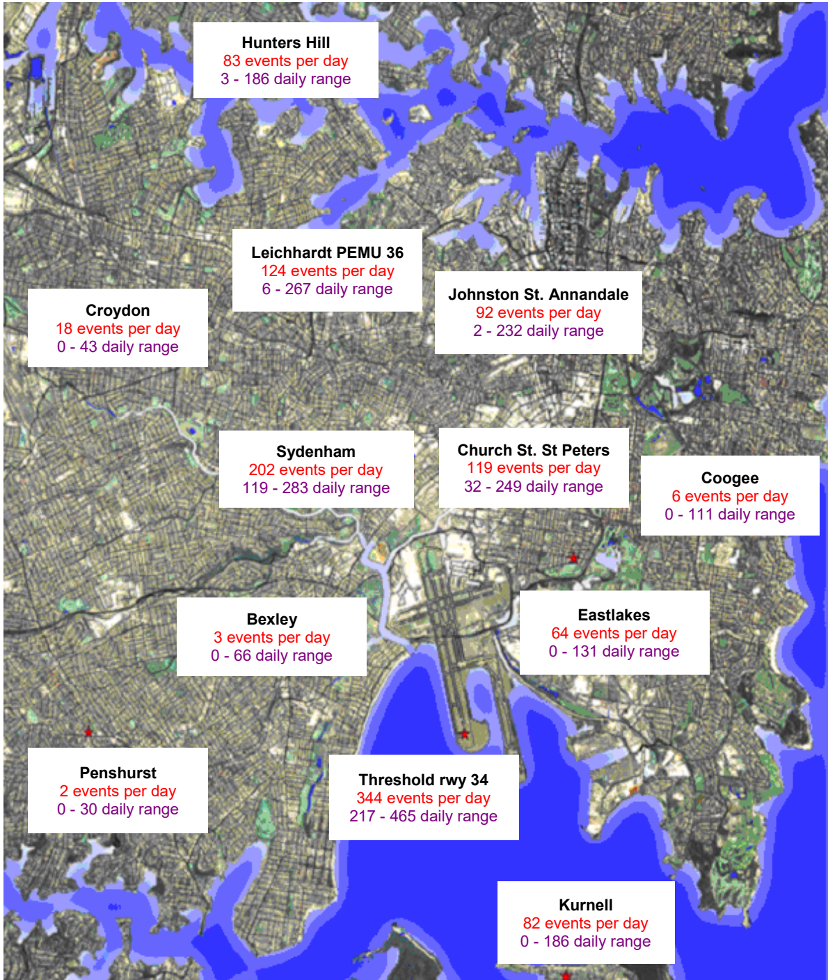
Figure 1. NMT sites about Sydney Airport and the daily N70 values for the month of February 2019
