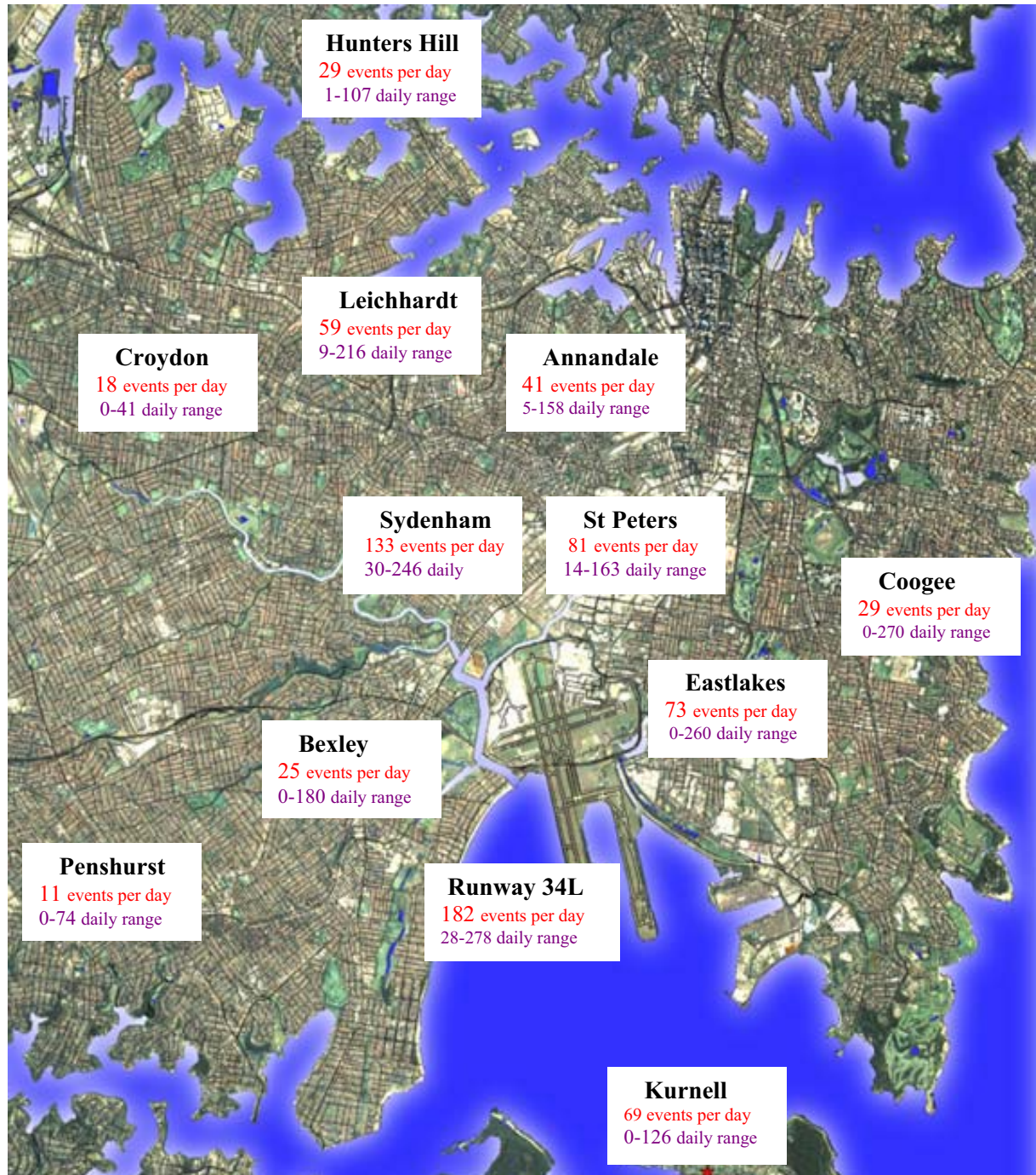
Figure 1. NMT sites about Sydney Airport and the daily N70 values for the month of September 2009
