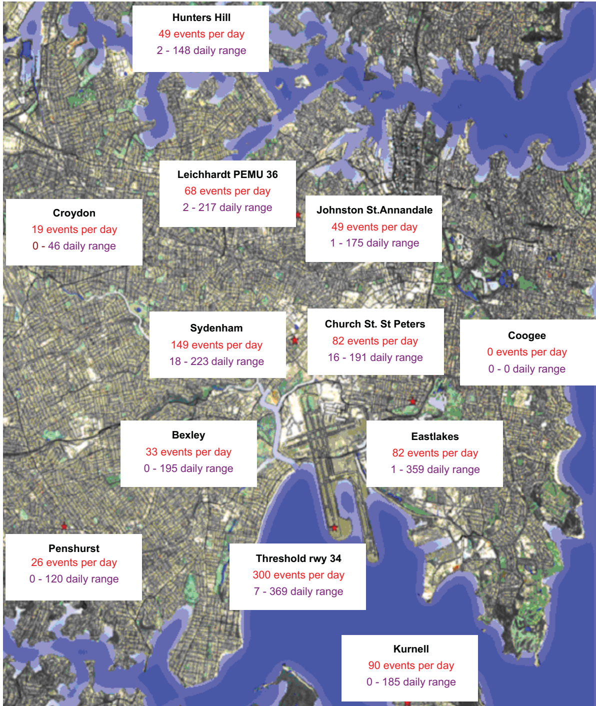
Figure 1. NMT sites about Sydney Airport and the daily N70 values for the month of October 2010
