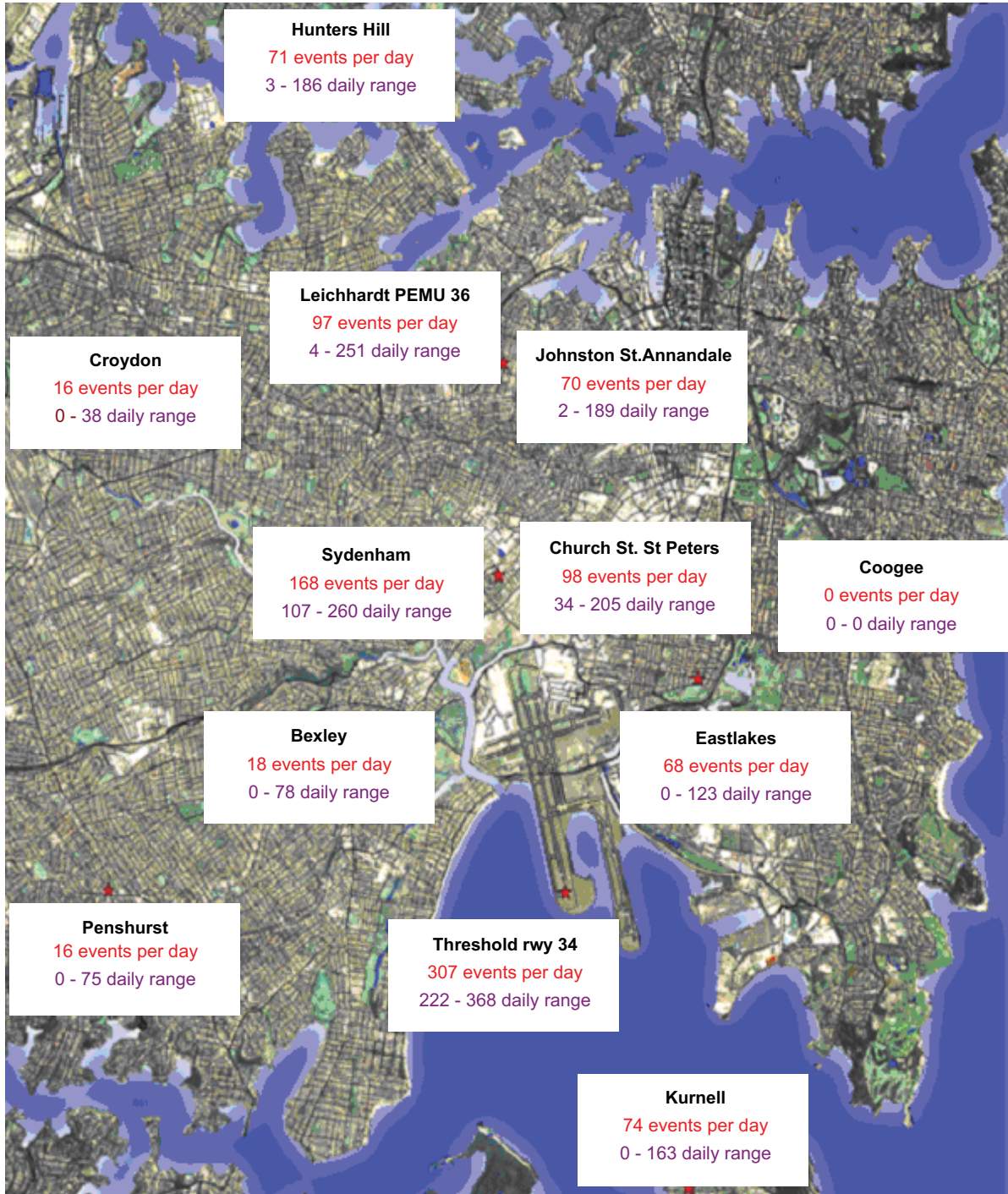
Figure 1. NMT sites about Sydney Airport and the daily N70 values for the month of November 2010
