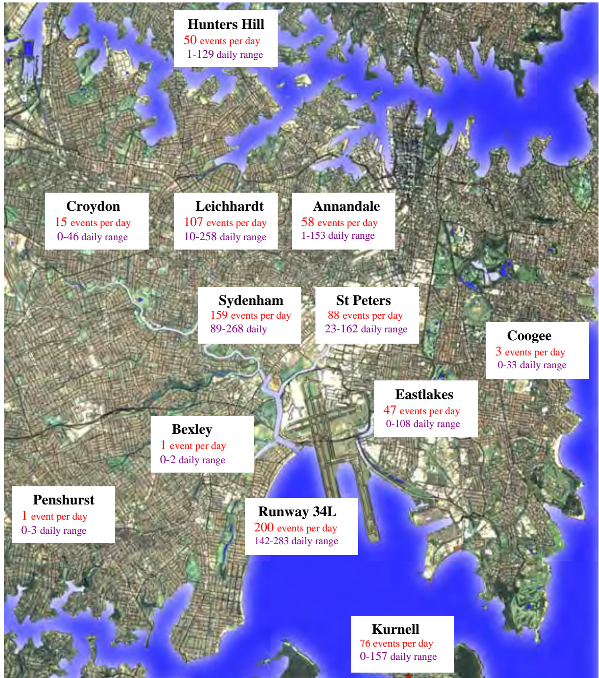
Figure 1. NMT sites about Sydney Airport and the daily N70 values for the month of November 2008
