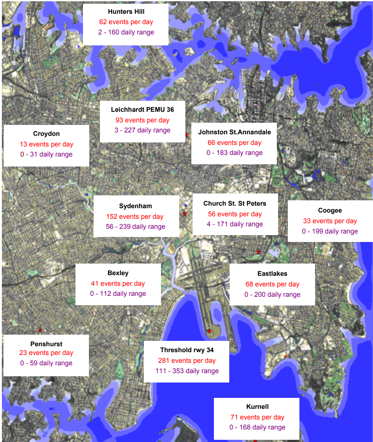
Figure 1. NMT sites about Sydney Airport and the daily N70 values for the month of May 2010
