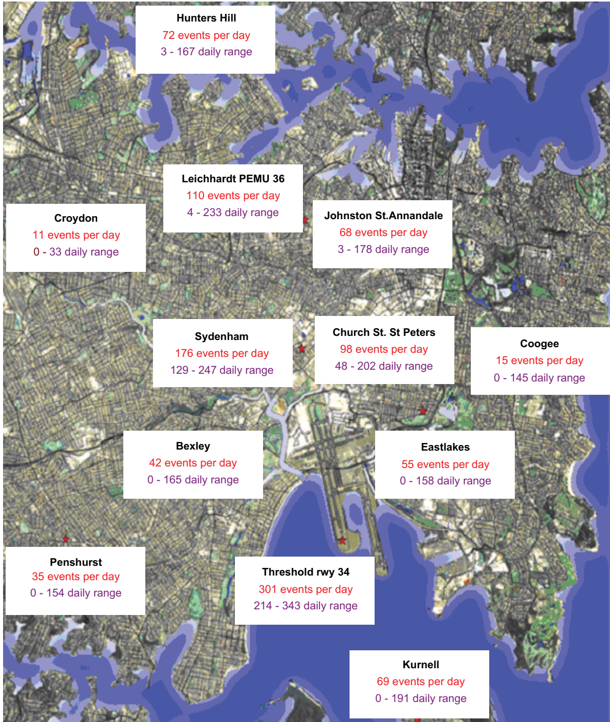
Figure 1. NMT sites about Sydney Airport and the daily N70 values for the month of March 2011
