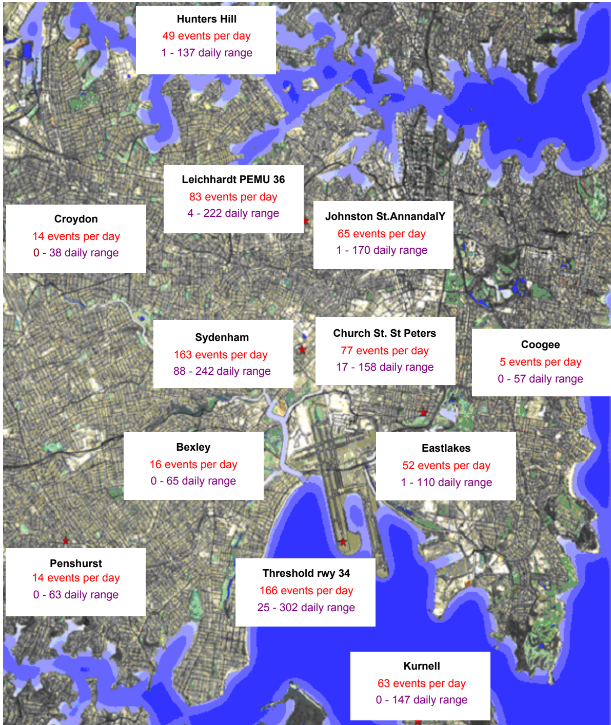
Figure 1. NMT sites about Sydney Airport and the daily N70 values for the month of March 2010
