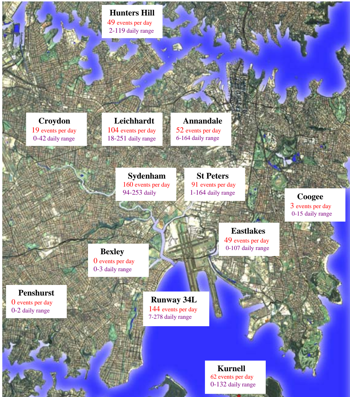
Figure 1. NMT sites about Sydney Airport and the daily N70 values for the month of March 2009
