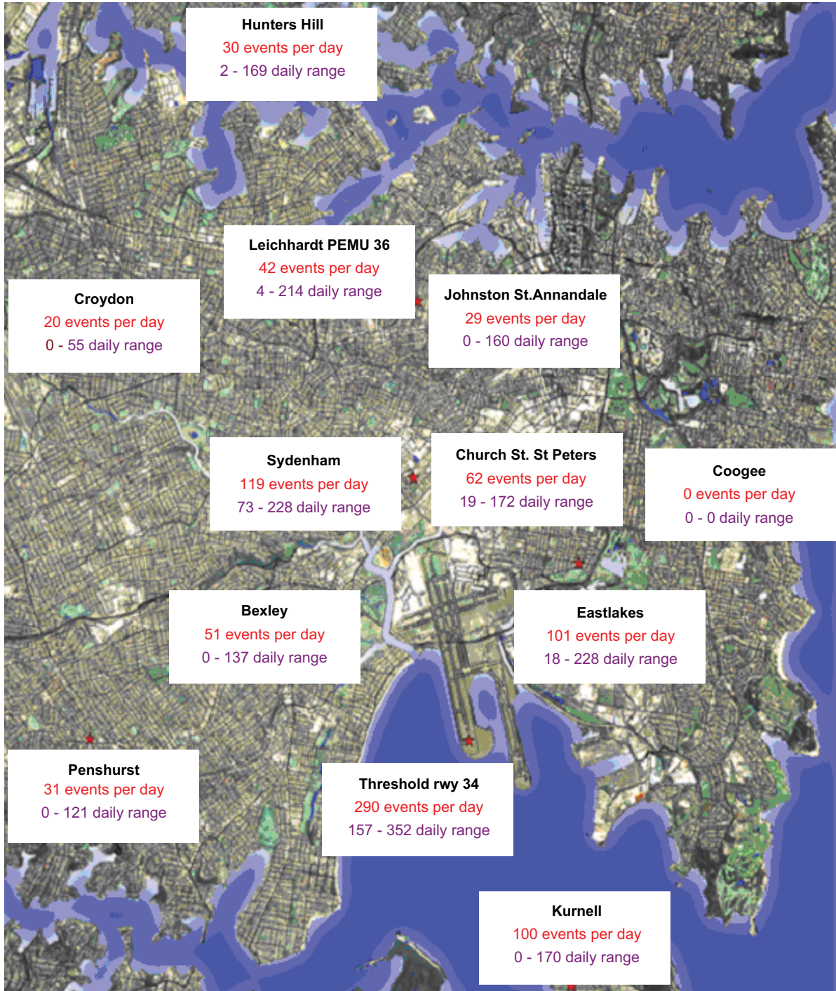
Figure 1. NMT sites about Sydney Airport and the daily N70 values for the month of August 2010
