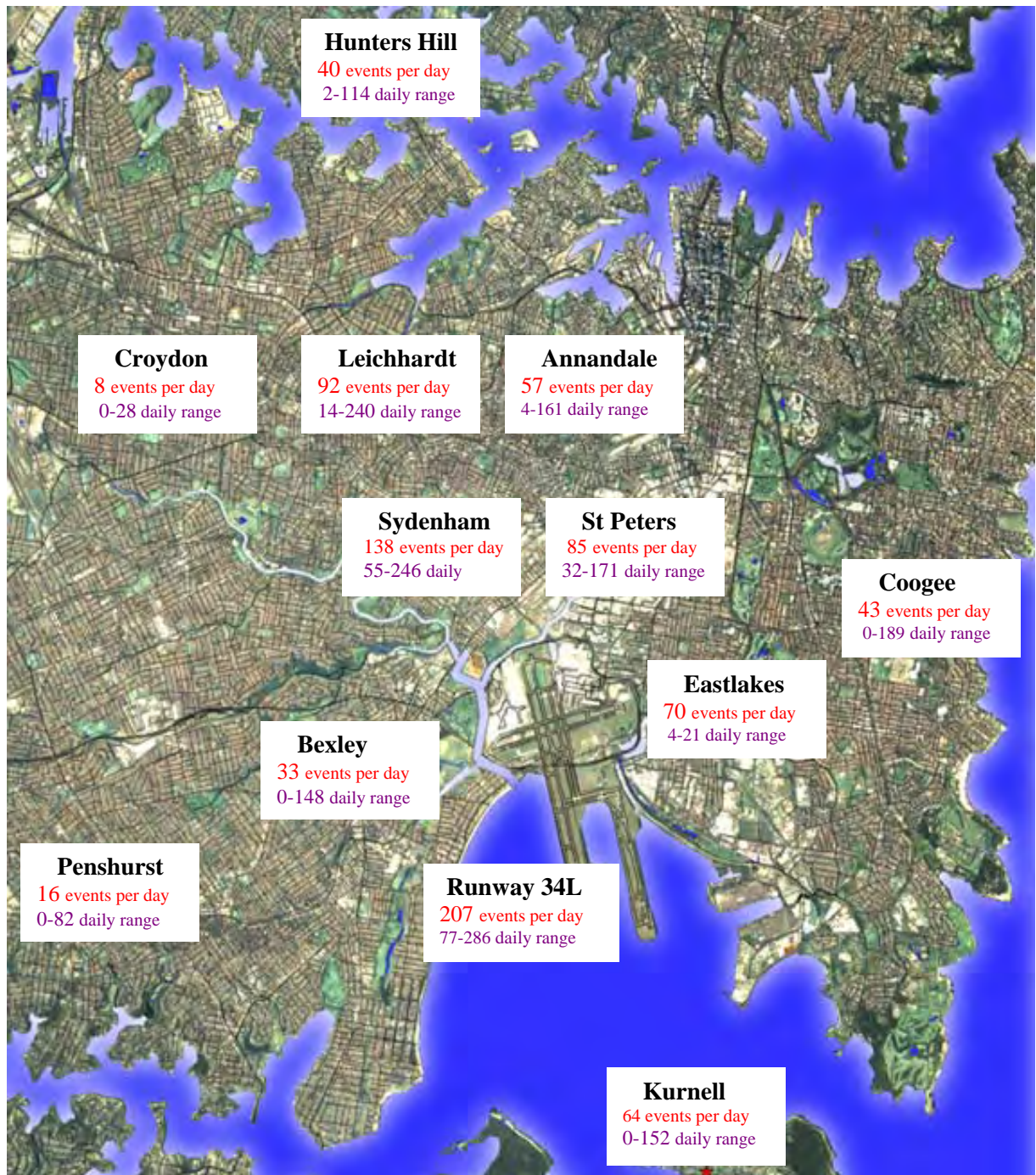
Figure 1. NMT sites about Sydney Airport and the daily N70 values for the month of August 2008.
