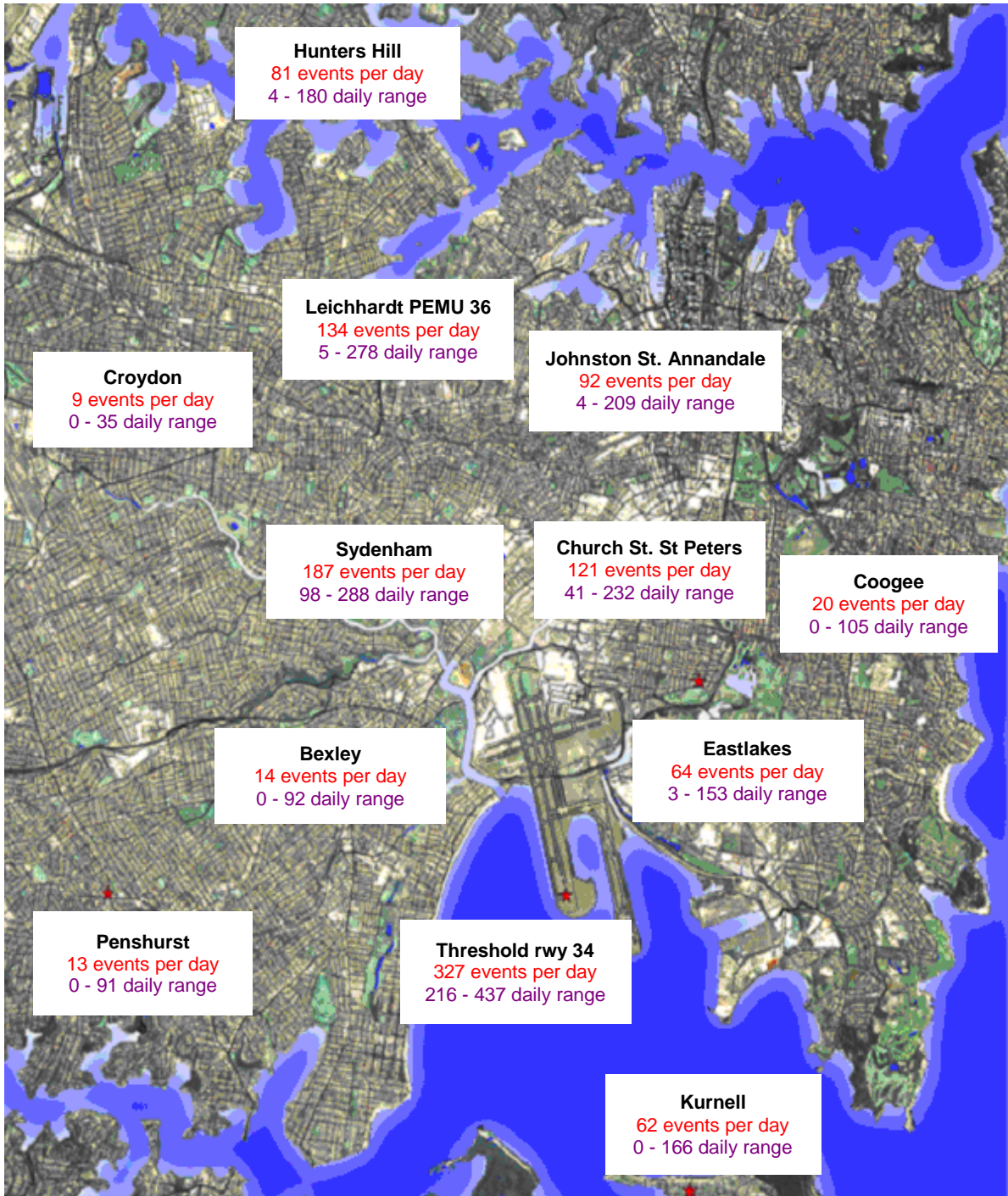
Figure 1. NMT sites about Sydney Airport and the daily N70 values for the month of September 2015
