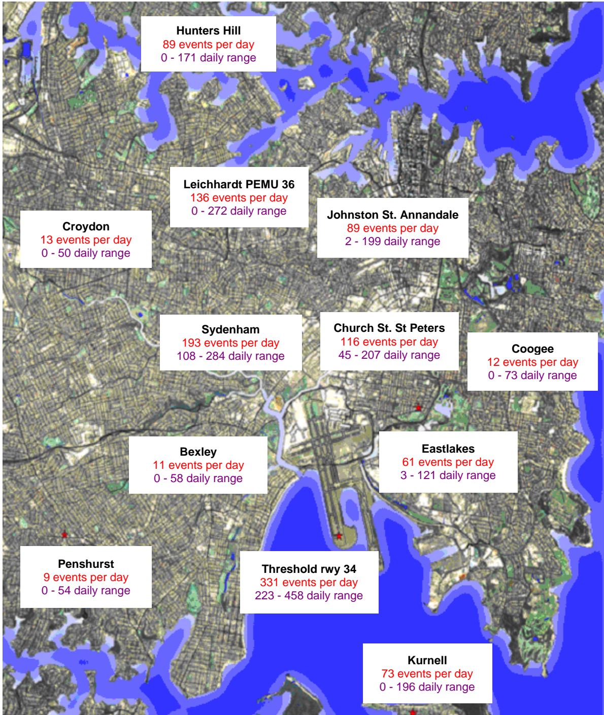
Figure 1. NMT sites about Sydney Airport and the daily N70 values for the month of September 2014
