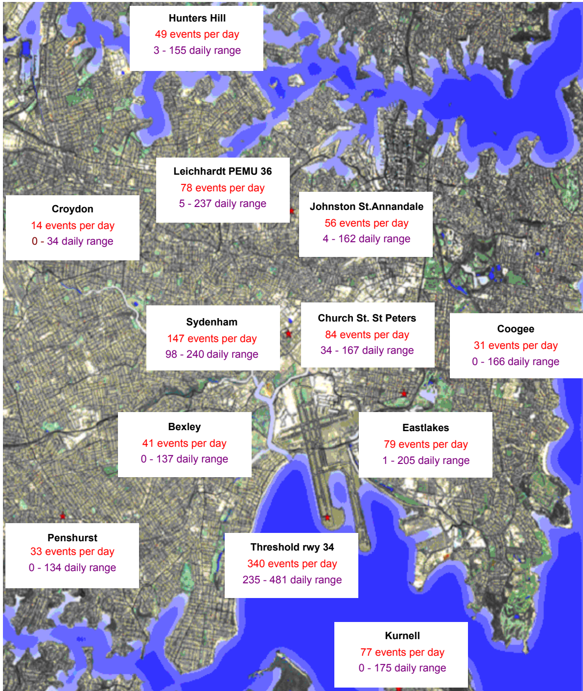
Figure 1. NMT sites about Sydney Airport and the daily N70 values for the month of September 2011
