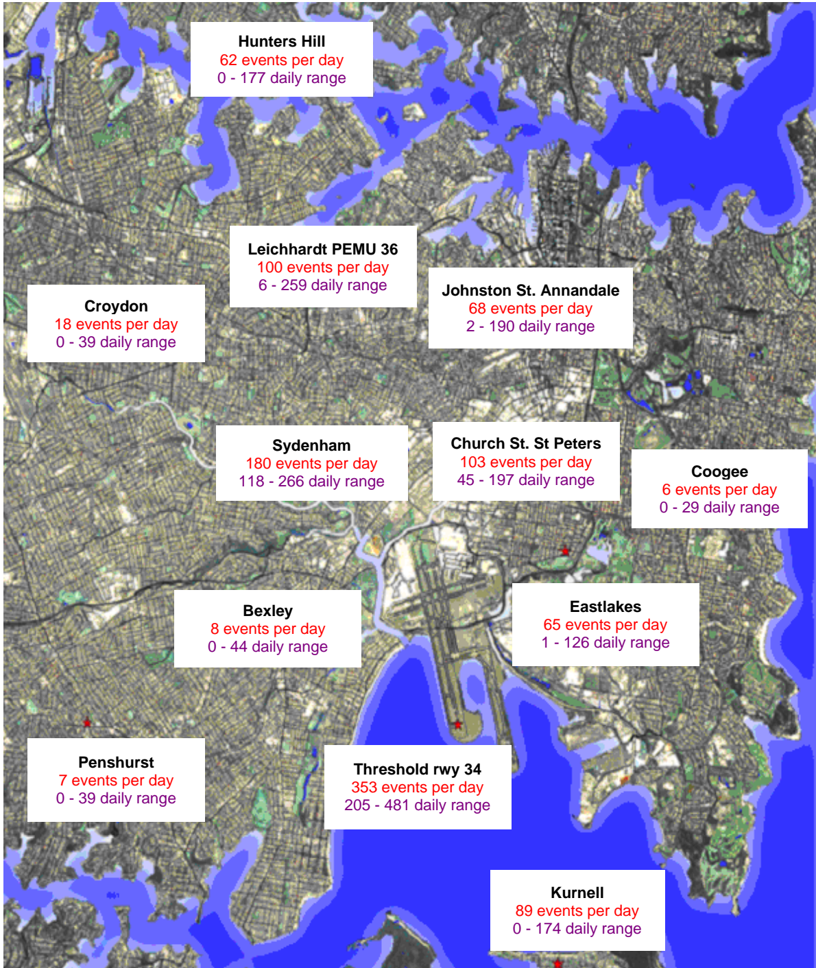
Figure 1. NMT sites about Sydney Airport and the daily N70 values for the month of October 2014
