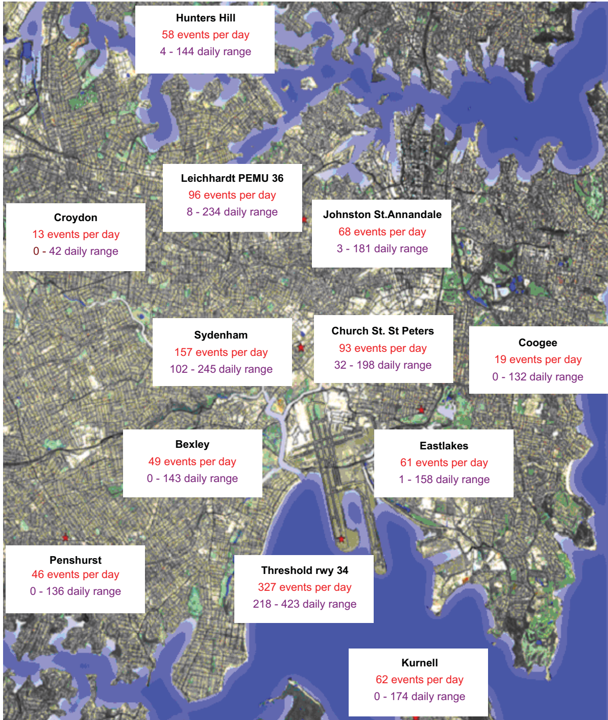
Figure 1. NMT sites about Sydney Airport and the daily N70 values for the month of October 2011
