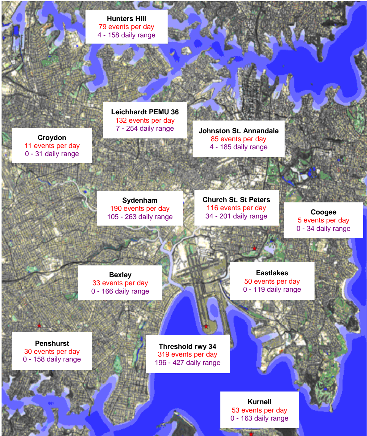
Figure 1. NMT sites about Sydney Airport and the daily N70 values for the month of March 2015
