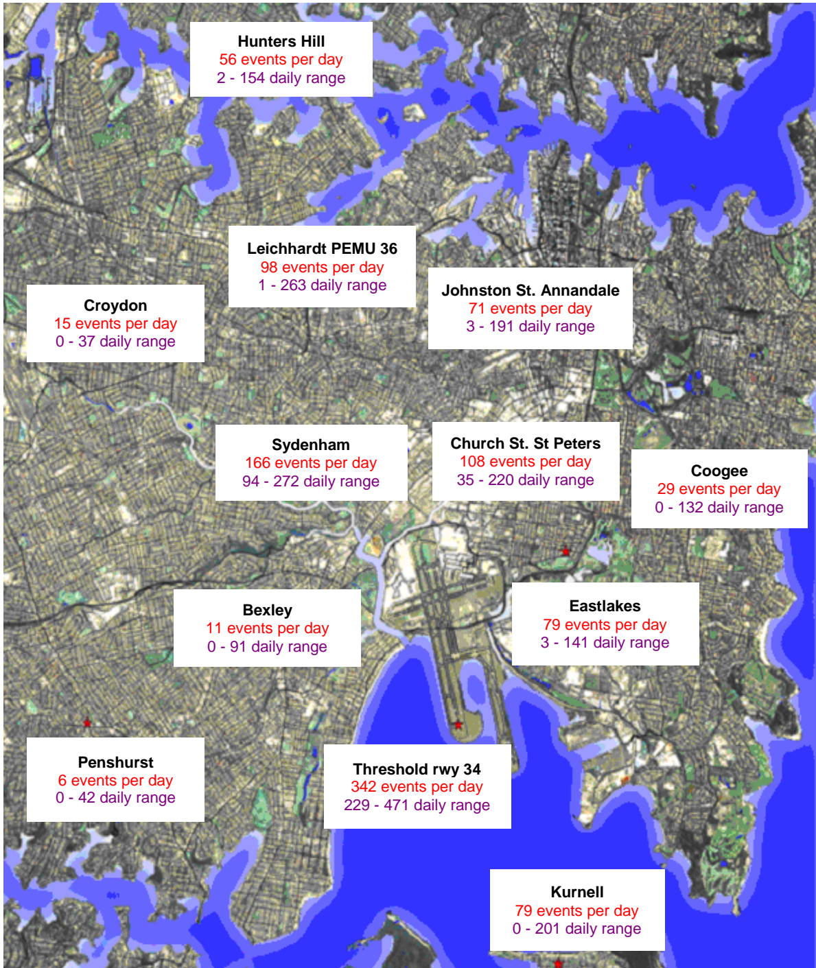
Figure 1. NMT sites about Sydney Airport and the daily N70 values for the month of June 2015
