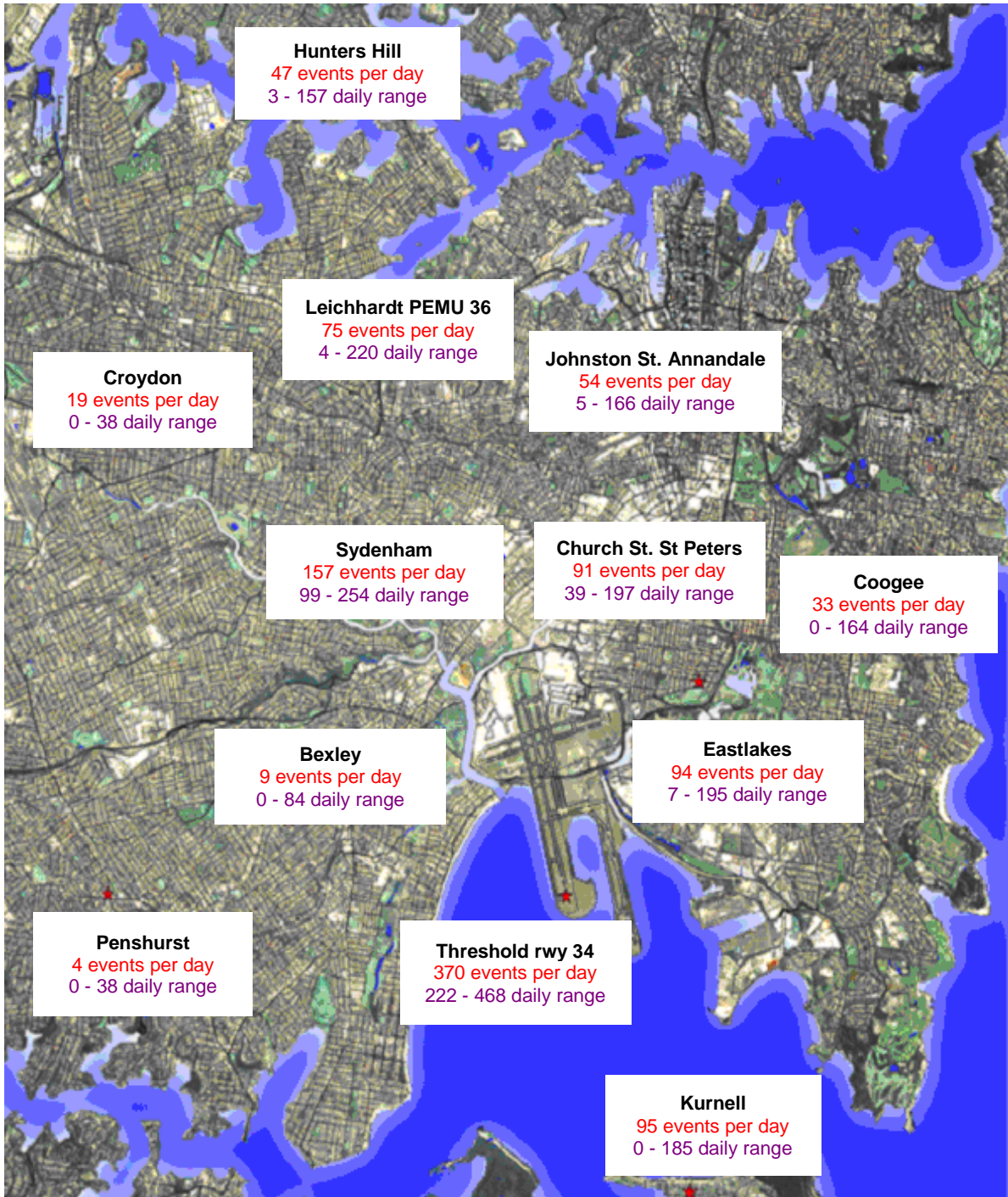
Figure 1. NMT sites about Sydney Airport and the daily N70 values for the month of July 2015
