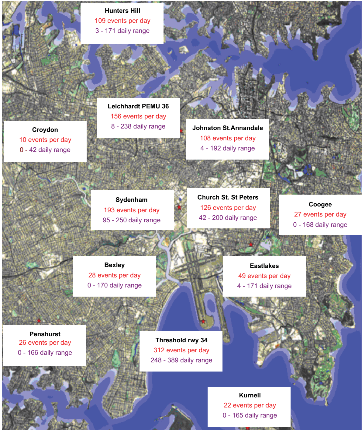
Figure 1. NMT sites about Sydney Airport and the daily N70 values for the month of December 2011
