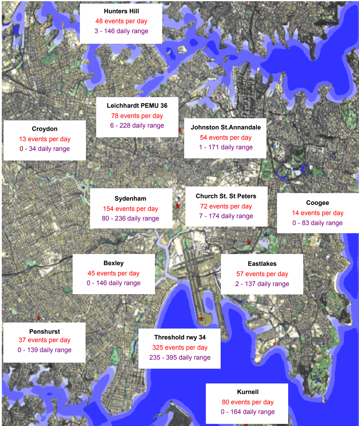
Figure 1. NMT sites about Sydney Airport and the daily N70 values for the month of August 2011
