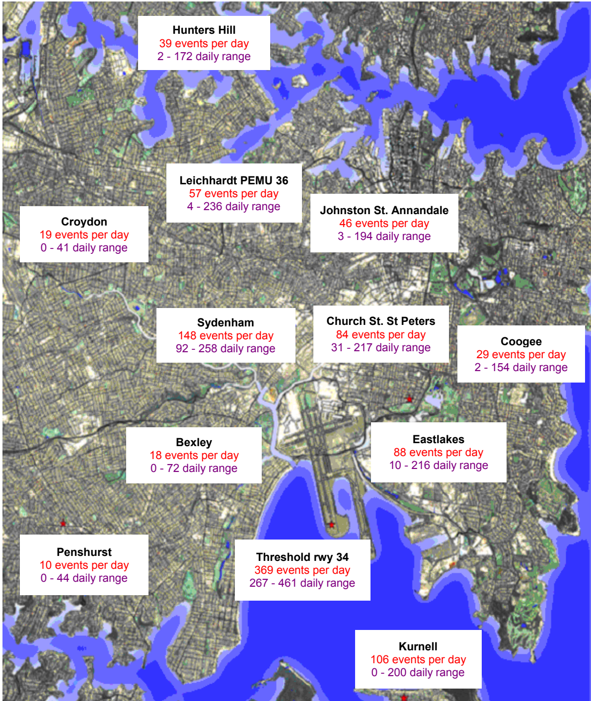
Figure 1. NMT sites about Sydney Airport and the daily N70 values for the month of August 2013
