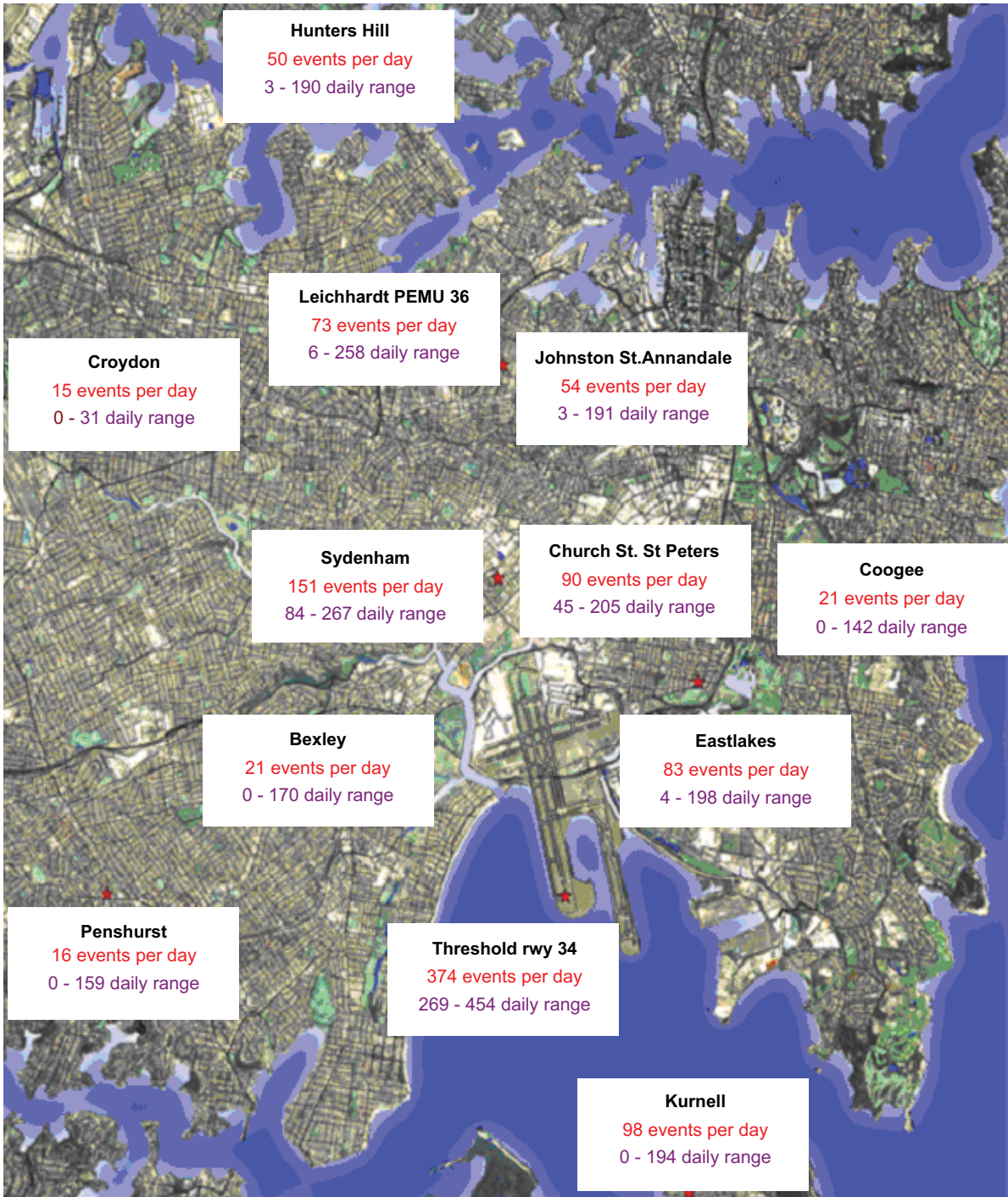
Figure 1. NMT sites about Sydney Airport and the daily N70 values for the month of September 2012
