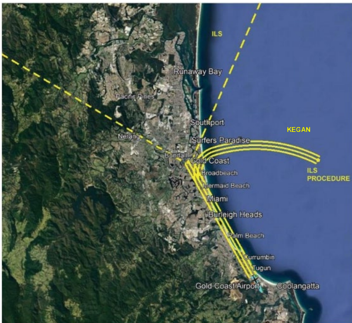
Figure 4: Flight paths used for the Airservices 2014 EIA, Source: Airservices Fact Sheet – Instrument Landing System for Gold Coast Airport
