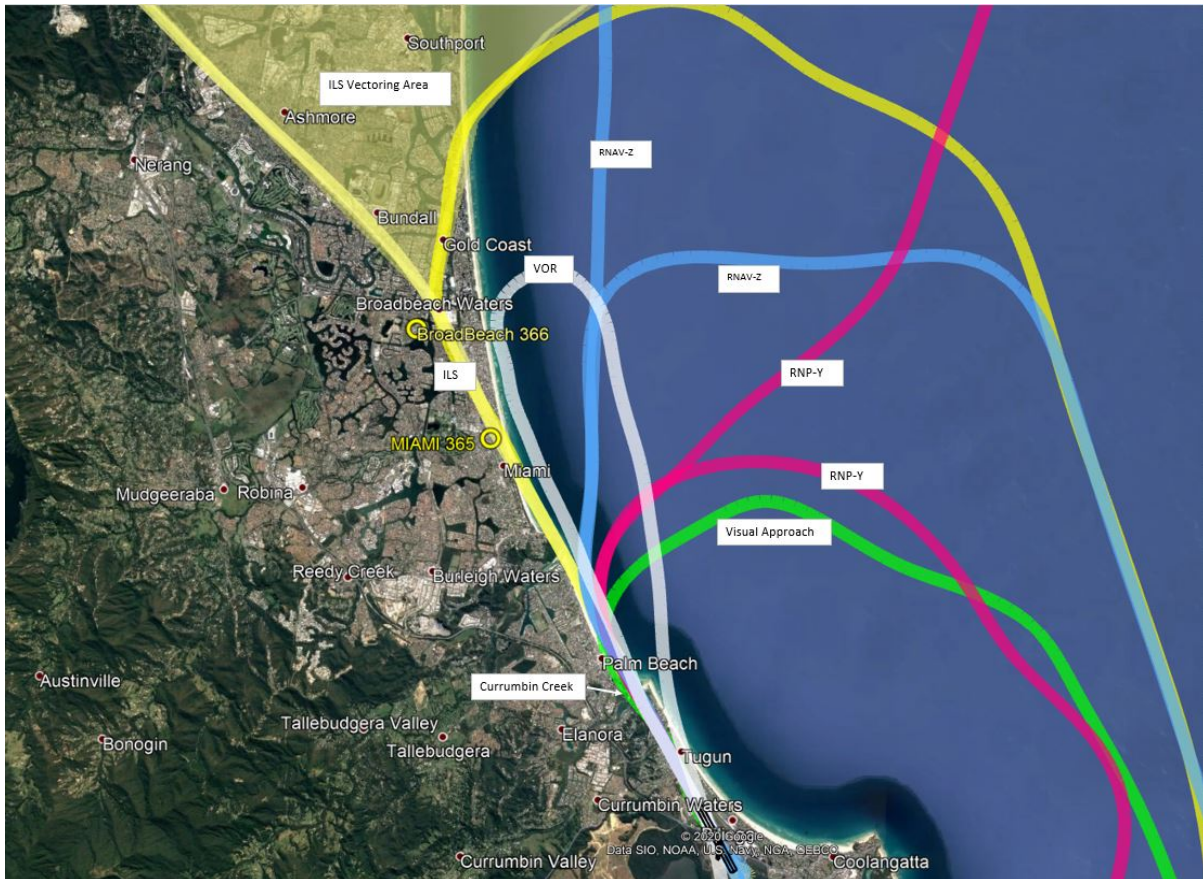
Figure 2: Depiction of current arrivals and approach procedures to RWY 14 at Gold Coast Airport, Source: Airservices NFPMS
