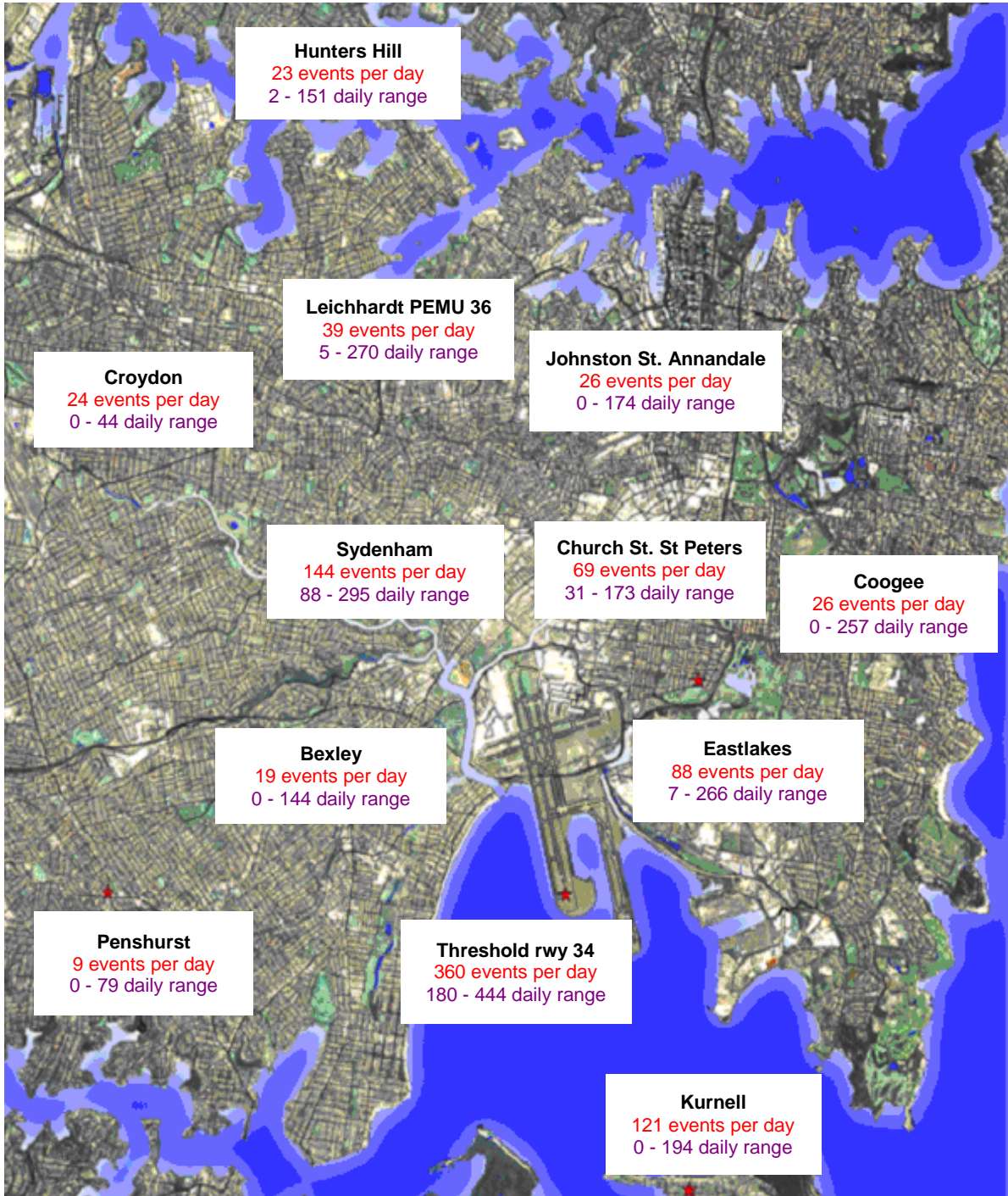
Figure 1. NMT sites about Sydney Airport and the daily N70 values for the month of May 2016
