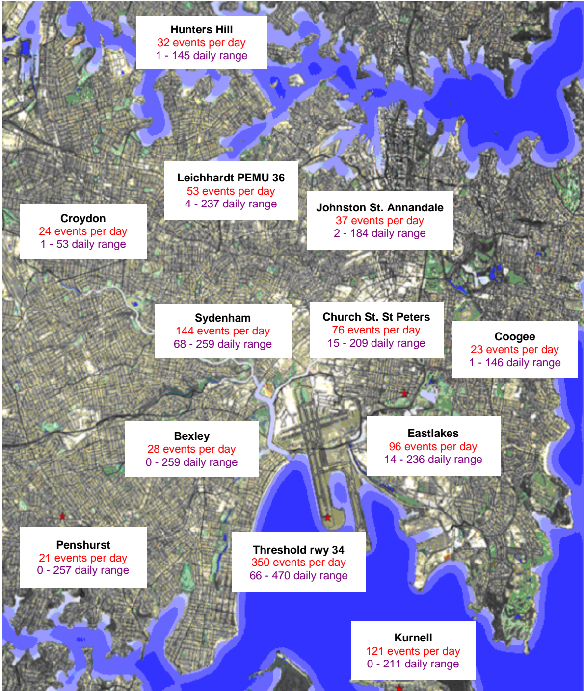
Figure 1. NMT sites about Sydney Airport and the daily N70 values for the month of June 2016
