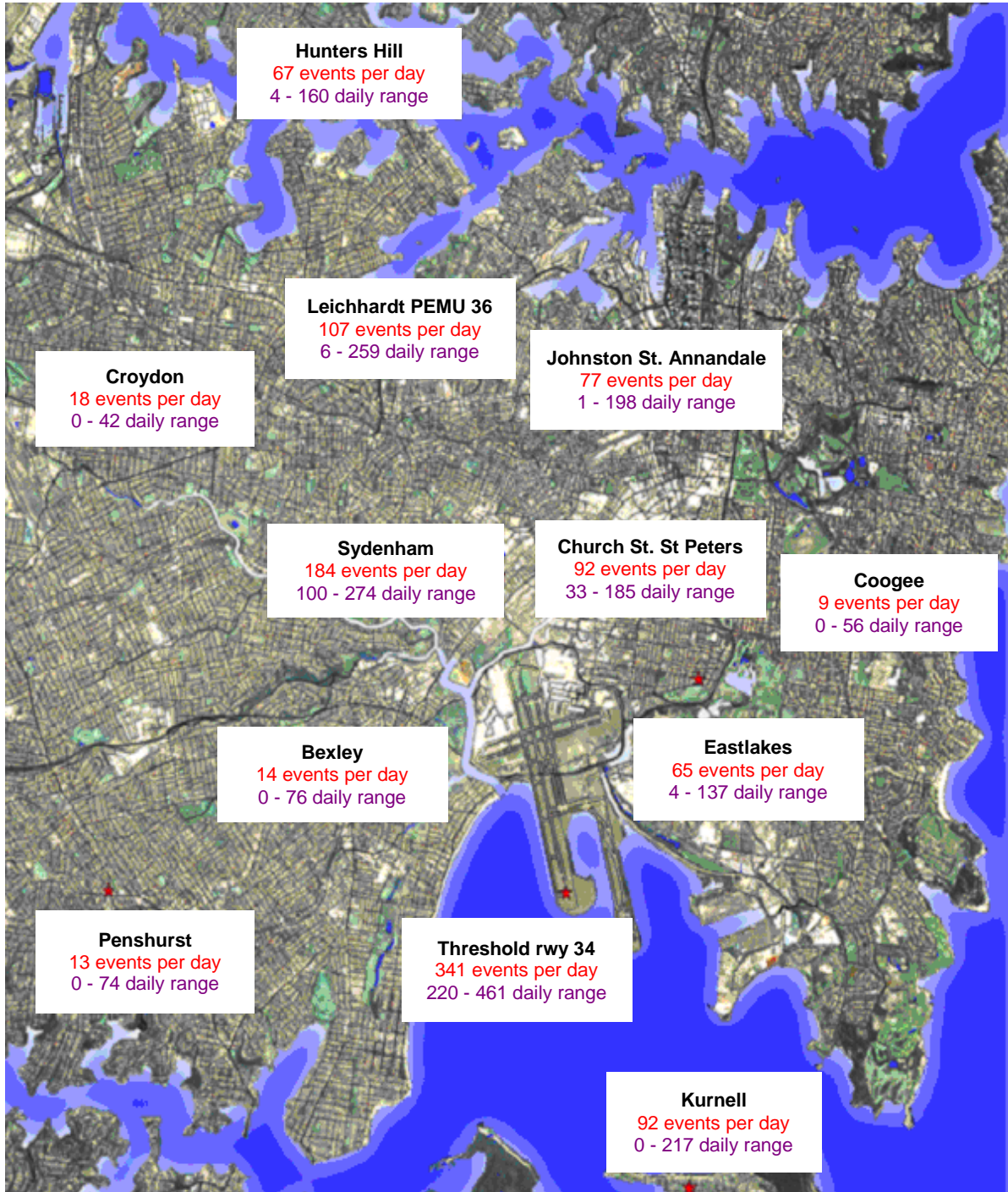
Figure 1. NMT sites about Sydney Airport and the daily N70 values for the month of April 2016
