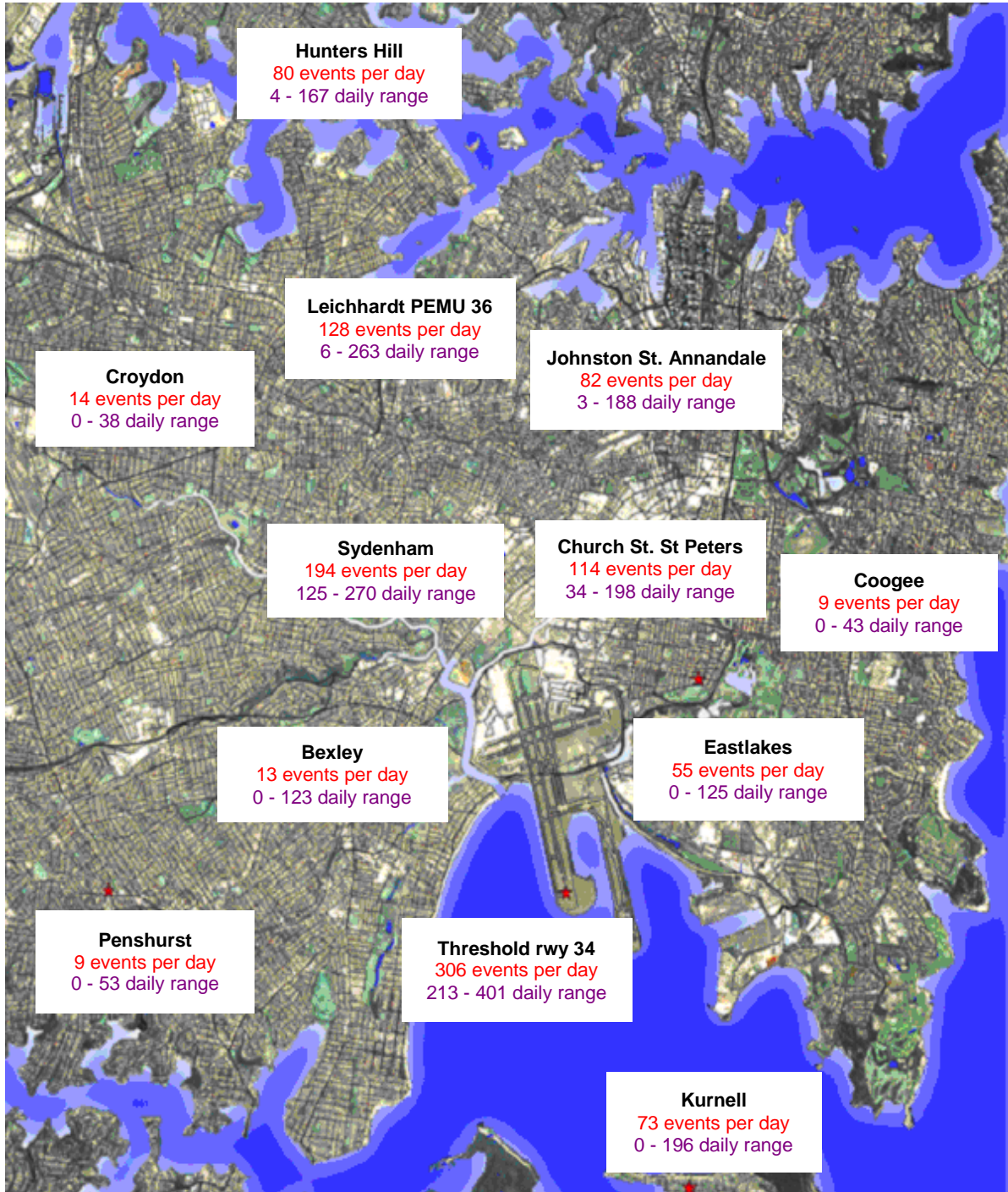
Figure 1. NMT sites about Sydney Airport and the daily N70 values for the month of January 2016
